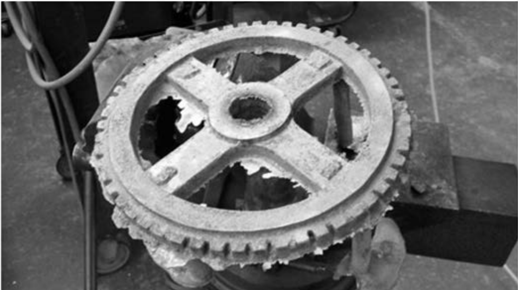
Figure 6. The directional gear in rough stage. Needs significant grinding but the overall shape looks good.
