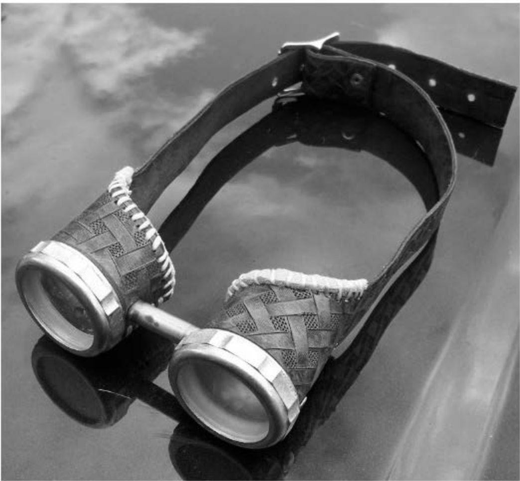
Figure 17. Completed goggles with nosepiece and buckle attached. These pieces only used one rivet.
