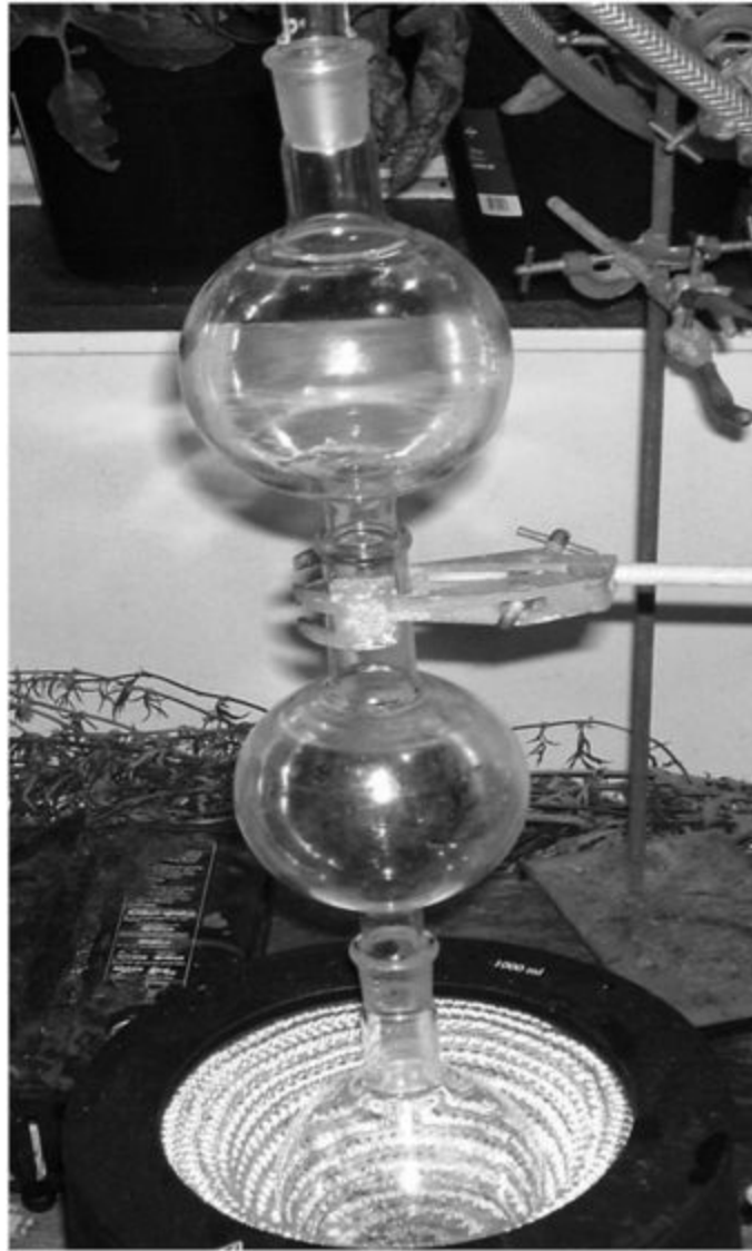
Figure 13: Two aludels working together. These will need to be made to order
