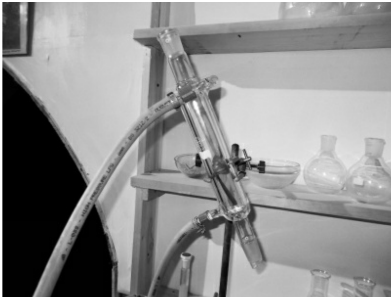
Figure 6: Condenser: cold water enters at the bottom and exits at the top
