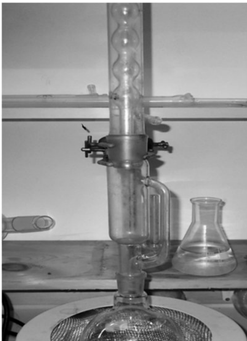
Figure 7: Soxhlet: condenser fits on the top of the soxhlet
