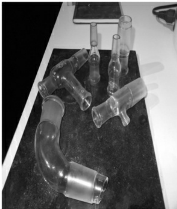
Figure 10: Joints allowing different size glassware to connect
